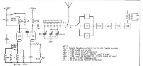
Fig. 1. The Tx/Rx circuit (simplified).
