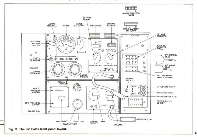
Should you reach 0 on either of the two tuning controls while tuning, then use a higher frequency coil. For example, if you are using L3A and the control reaches 0, then use L3B. Should you reach 10 on either coil then use a lower frequency coil.
