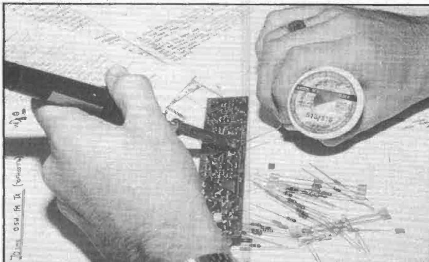
Fitting a tiny 82pF capacitor into the correct holes in the PCB.
