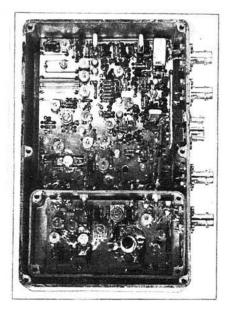
(basic sensitivity  $0.2\mu V$ ) the transverter produced a 12dB SINAD figure at  $0.12\mu V$  p.d.
