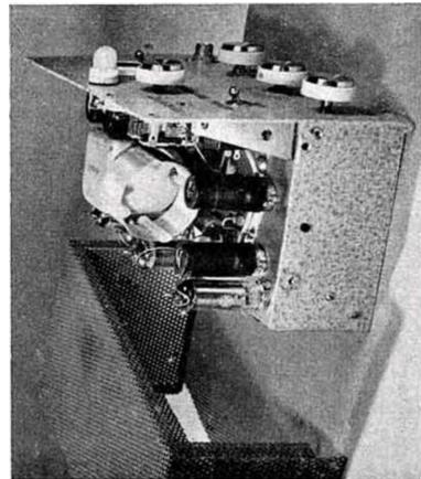
Three-quarter view of the miniature Top Band transmitter and its perforated zinc cover. The large inductor visible just in front of the modulator transformer is the p.a. coil. A Codeur coil should be available.
