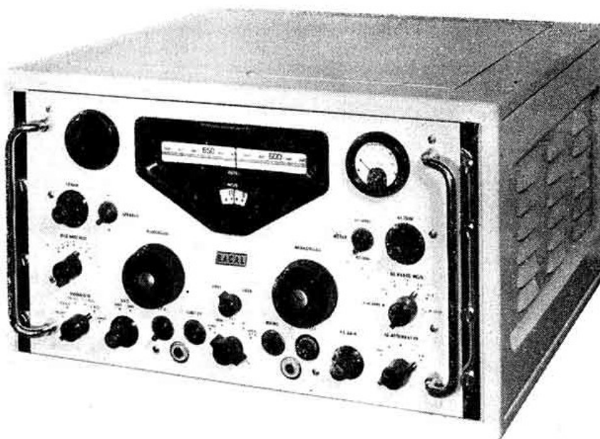
A front panel view of the Racal RA17 Receiver.
