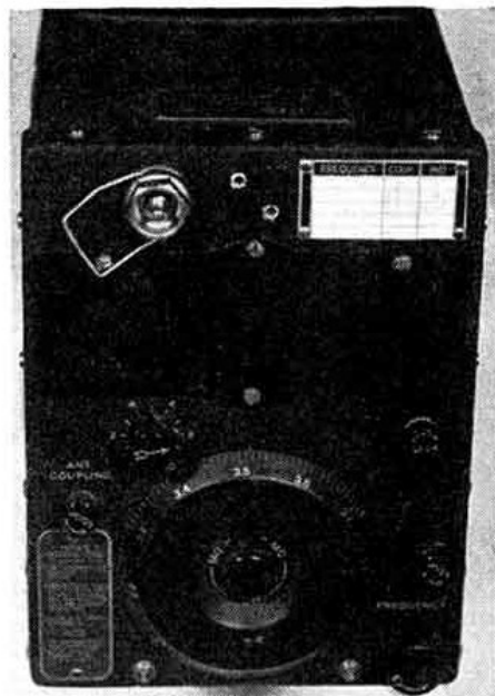
Front view of the transmitter after modification. Note the aluminium panel covering the "window" above the tuning dial.
