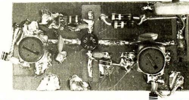
The alternative pre-amp design using a BF961 transistor and Toko coil formers with fixed tuning capacitors
